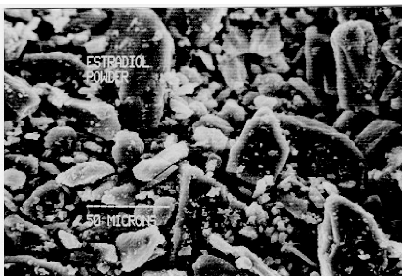
FIGURE 4 SEM Pictures of Beta-Estradiol Microparticles with PLGA 85/15 Biodegradable Polymer (A) and Beta-Estradiol Powder (B).
